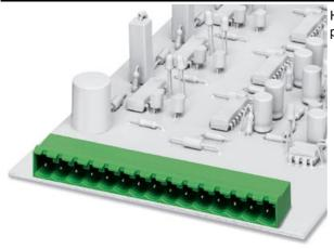
Header, nominal current: 12 A, rated voltage: 250 V, pitch: 5.08 mm, no. of positions: 11, mounting: Soldering
